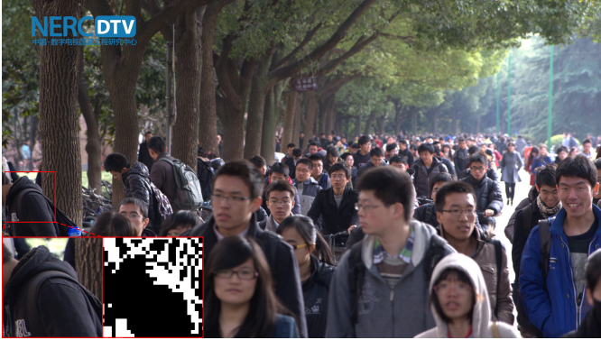
Fig. 4: Results of an interactive \times 2 zooming for a 4K image from the SJTU dataset (shown in the left red rectangle), accompanied by the upscaler decision mask (shown in the right red rectangle, black is bicubic and white is SR). Better viewed zoomed in.
